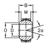
Α = 38 a (degrees) = 14 = 25 В D = 20 Dynamic load C (kN) = 78= 18 M 0 = 24.3
